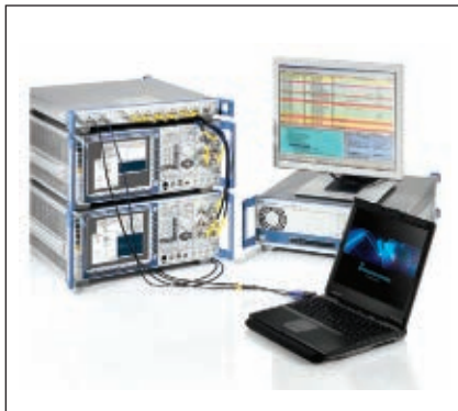
▲ Fig. 7 Multi-CMW setup for testing carrier aggregation mobility with 2x2 MIMO.
